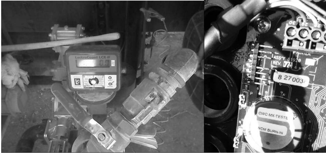
Figure 3 - Flow Meter Mounted onto Delivery Truck (Left) and the Hardware Interface (Right) Into the Laptop Computer
