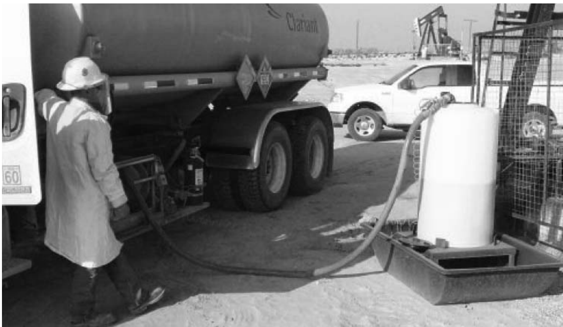
Figure 1 - Typical Operation During a Chemical Delivery to a Continuous Injection Well
