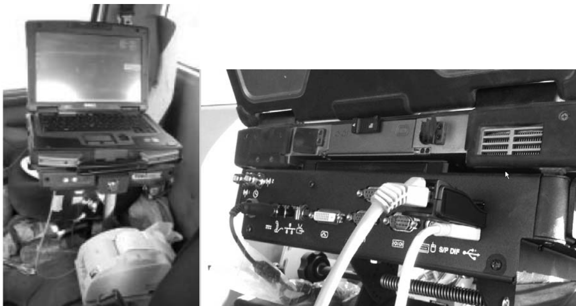
Figure 2 - Rugged Laptop Computer Mounted in the Cockpit of the Delivery Truck Front View (Left) And Rear View (Right)
