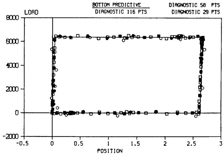
Figure 3 - Diagnostic pump cards vs points used
