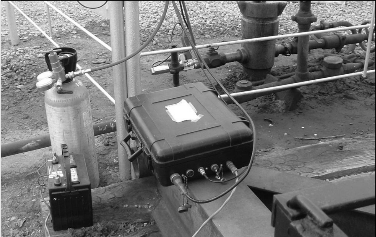
Figure 1 – Acoustic Liquid Level Set-Up for Programmed Automatic Operation
