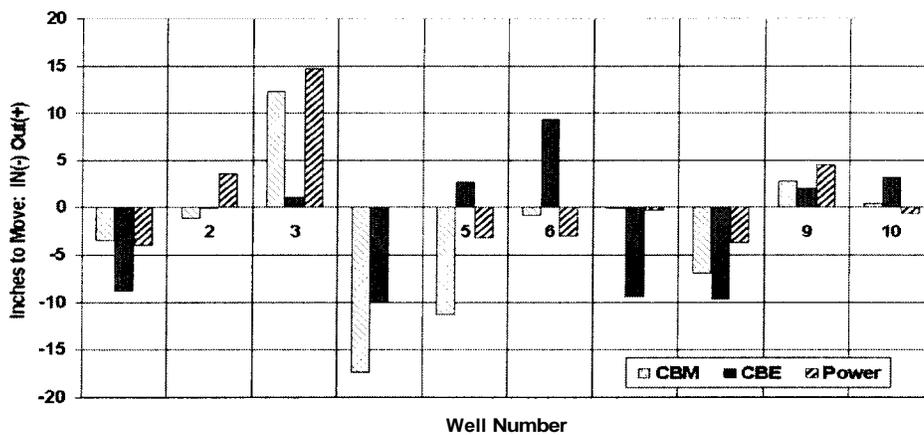
Figure 8 - Move Counterweights from Current Position for Wells 1-10
