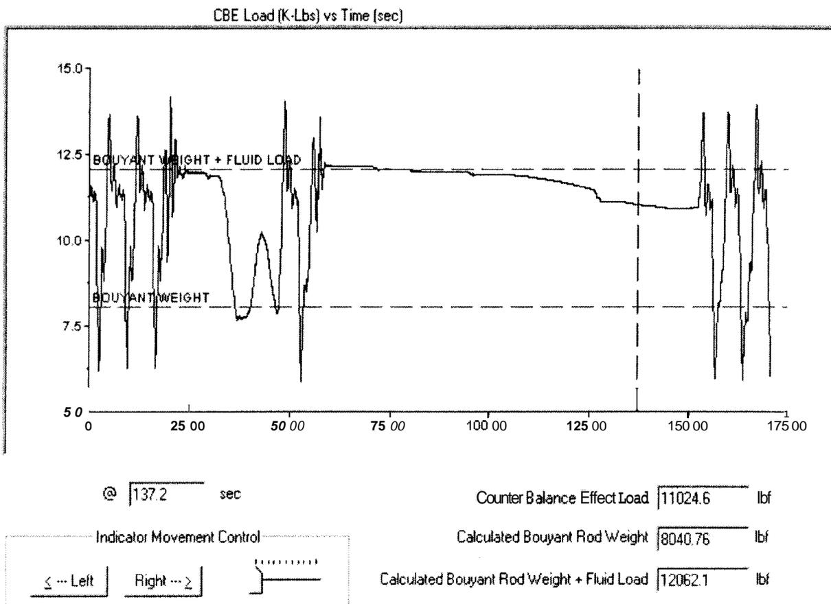
Figure 7 - Counterbalance Effect Test
