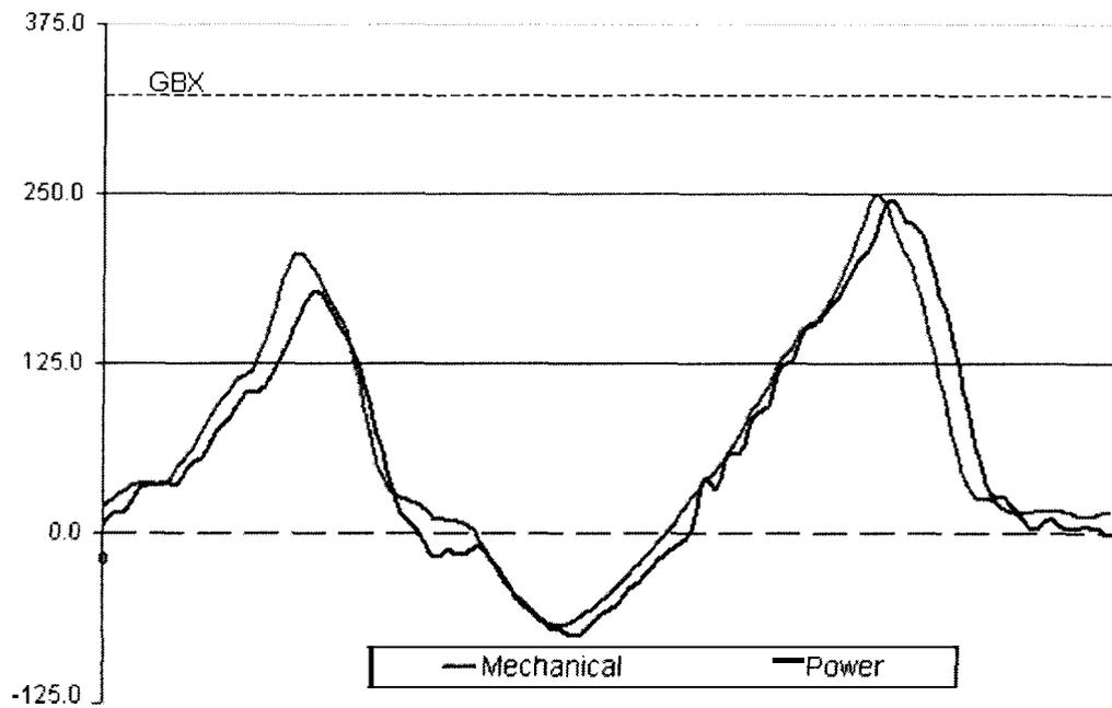
Figure 2 - Compare Motor Output Torque and Gearbox Torque
