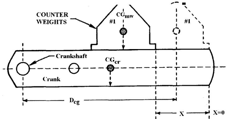
Figure 5 - Conventional Pumping Units with Crank Mounted Counterweights
