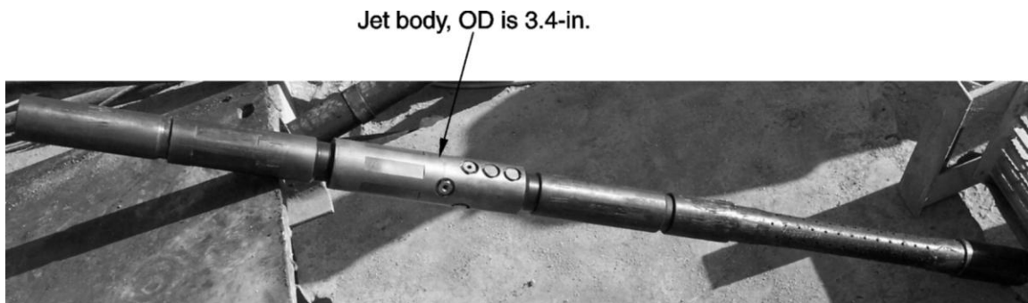
Figure 2—BHA used on recent jointed tubing hydrajct-fracturing treatment in western Asia.
