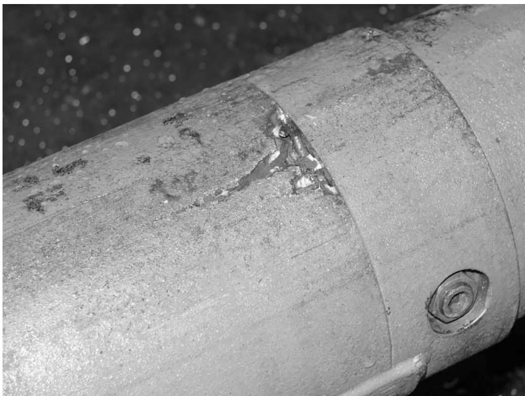
Figure 1-4: More corrosion on the same ESP.
