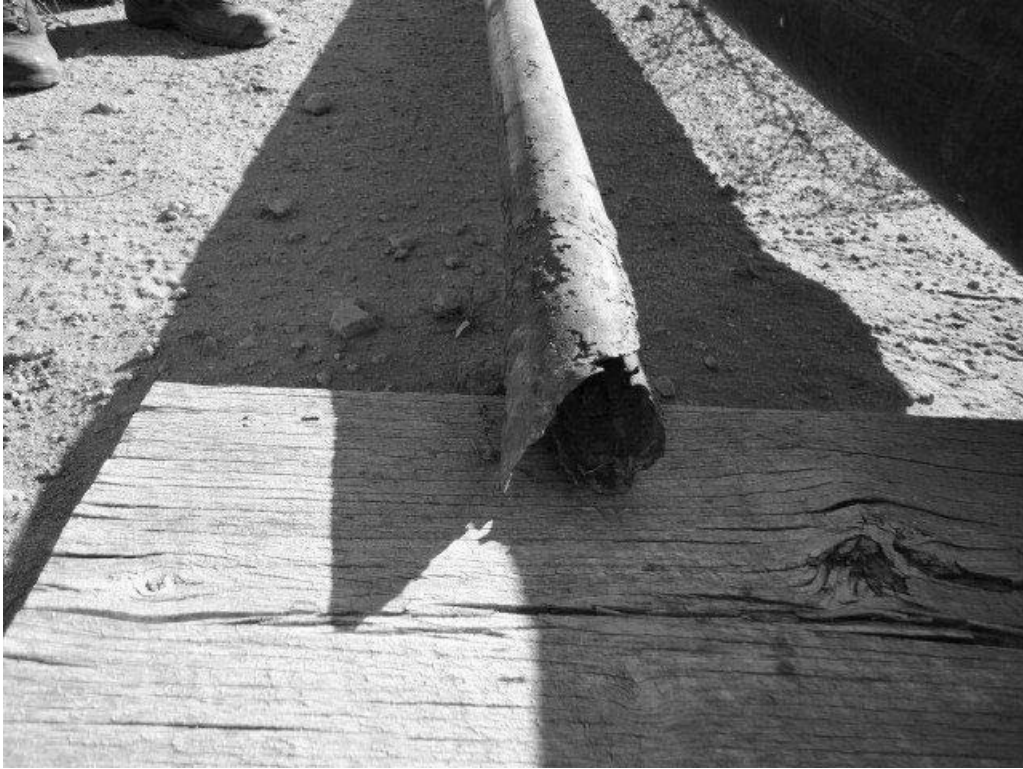
Figure 1-1: Example of bare steel tubing after six weeks
