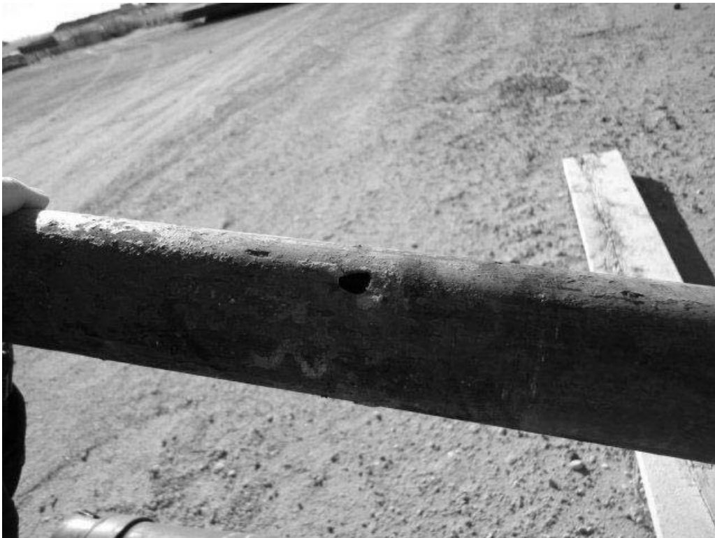
Figure 1-2: Hole in IPC tubing. A regular occurrence at Postle.
