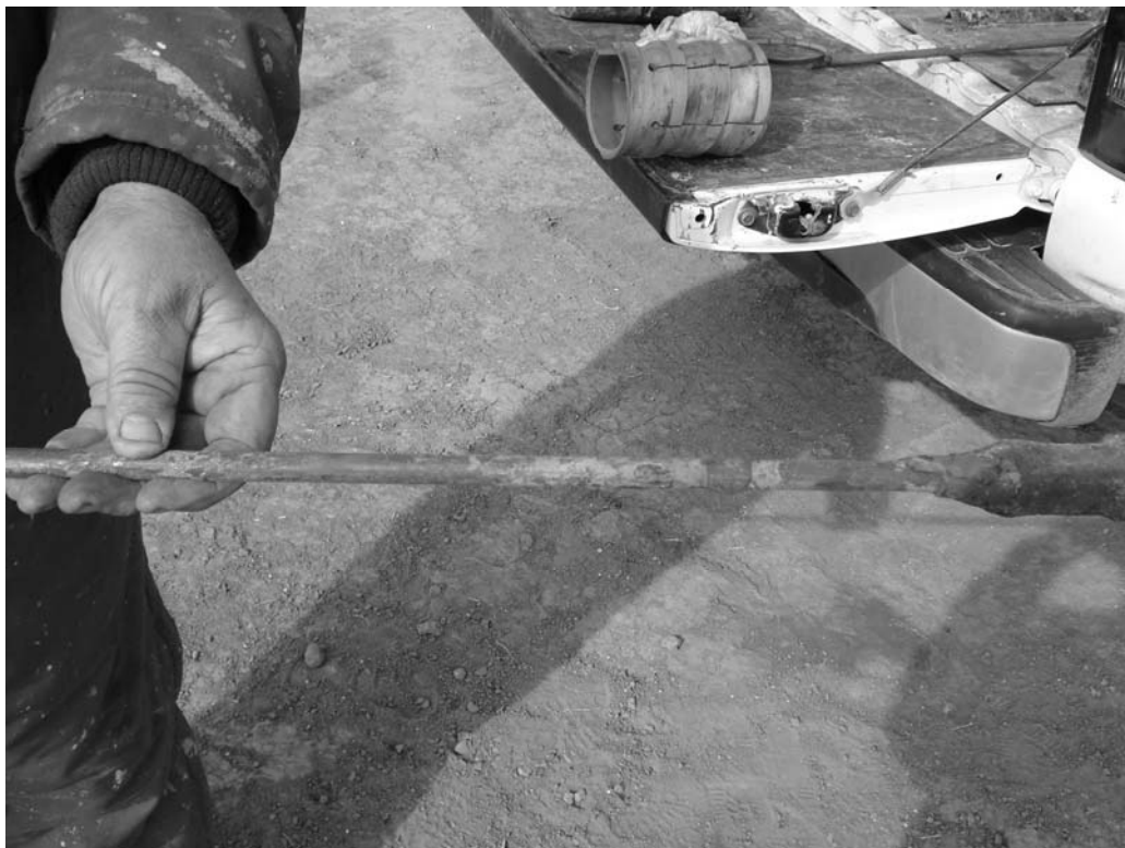
Figure 2-4: \frac{3}{4} " steel rod with severe corrosion and pitting
