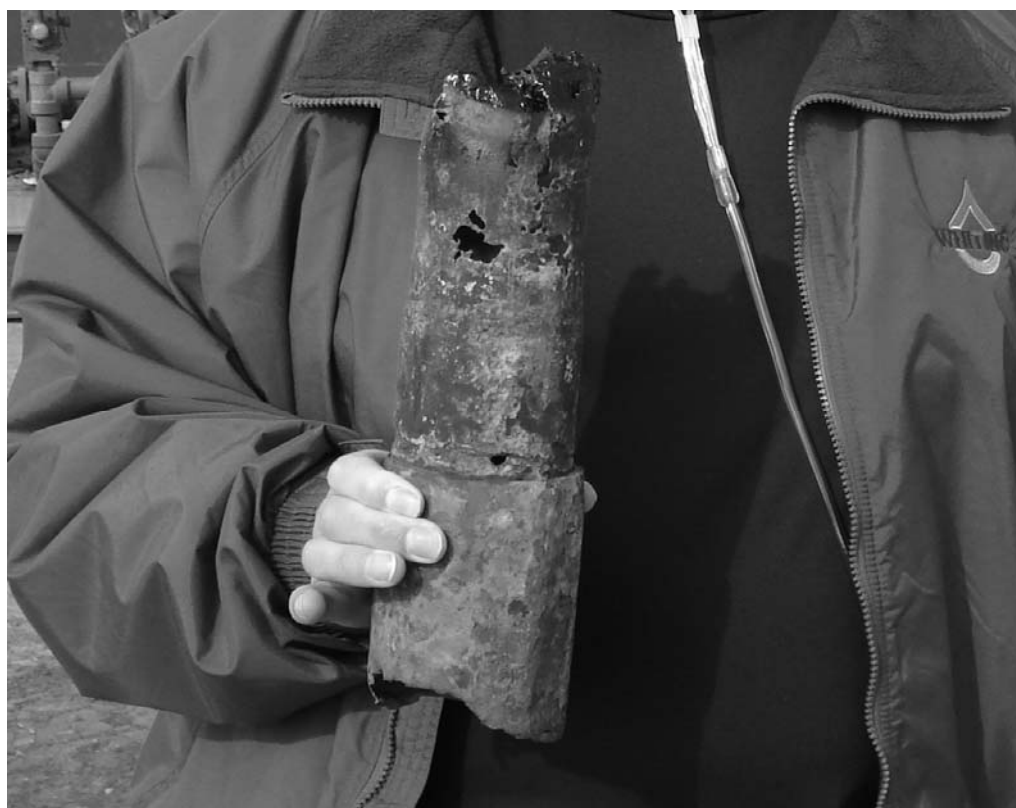
Figure 2-5: Corroded 2-7/8" collar. Paper thin wall with pits and holes.
