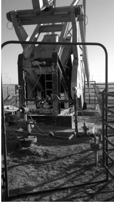
Figure 4-1: "Poor-Boy" Gas Lift assembly at the wellhead. 3/8" stainless steel capillary string is connected to a CO 2 supply line from the nearest injector. Gas lift has been able to replace many pumping units at Postle.
