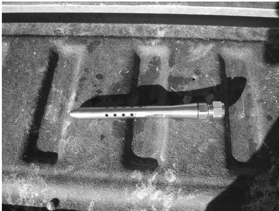
Figure 4-2: Check valve that is installed at the end of the capillary string 4500 feet down in the tubing
