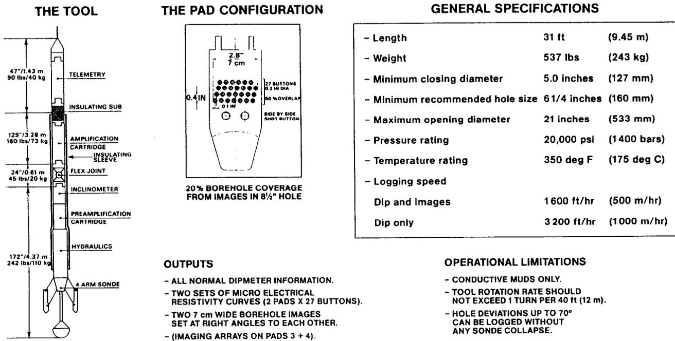
Figure 1 - The tool — technical specifications
