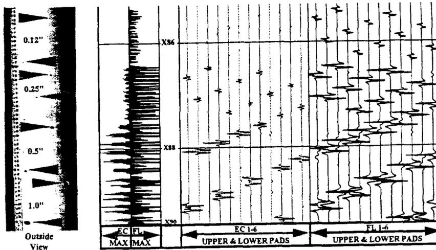
Log Example #2: The example above is from a section of test casing with man-made thru-hole defects. A photograph of the outside of the pipe is shown next to the log and scaled to match the scale of the log presentation.
