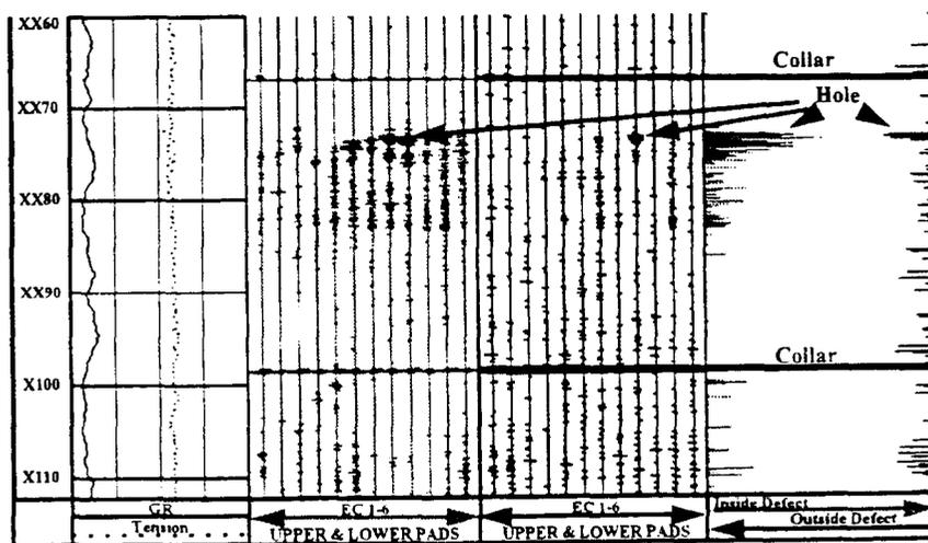
Log Example #4: The example above is from a well in West Texas in a 7.9" 20#/ft. pipe. The casing profile in the far right track is a discriminated maximum defect from the inner and outer portions of the pipe.
