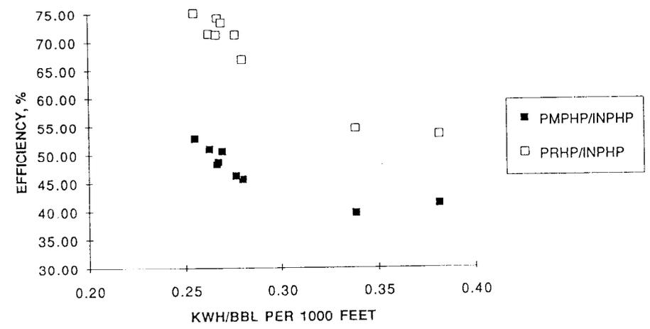
Figure 13 - Efficiencies for well in Figure 7.
