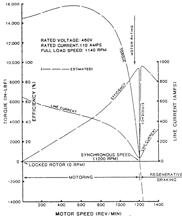
Figure 1 - Performance curves for a 100 HP NEMA-D motor (after Gibbs, SPEPE August 1987)
