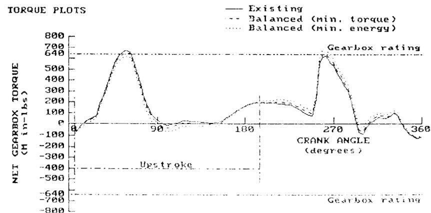
Figure 6 - Effect of direction of rotation on dynamometer and torque curves
