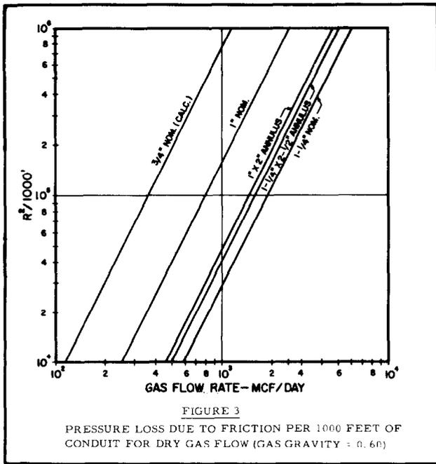
outlined by the Texas Railroad Commission.<sup>6</sup> The two curves for the small annuli indicate approximately the same pressure loss because the 1-in. tubing was non-upset (1,660-in. OD coupling) and the 1-1/4-in. tubing was upset (2,200-in. OD coupling). The term "R<sup>2</sup>" is a function of the pressure loss due to friction only and is used to calculate the downstream pressure (P<sub>dn</sub>) with the following equation:
