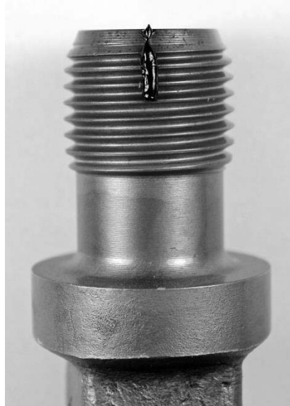
Figure 5 – example of applied thread lubricant.
