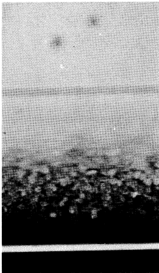
FIG. 5—TWO LB PER GAL. OF 10-20 MESH SAND IN WATER
