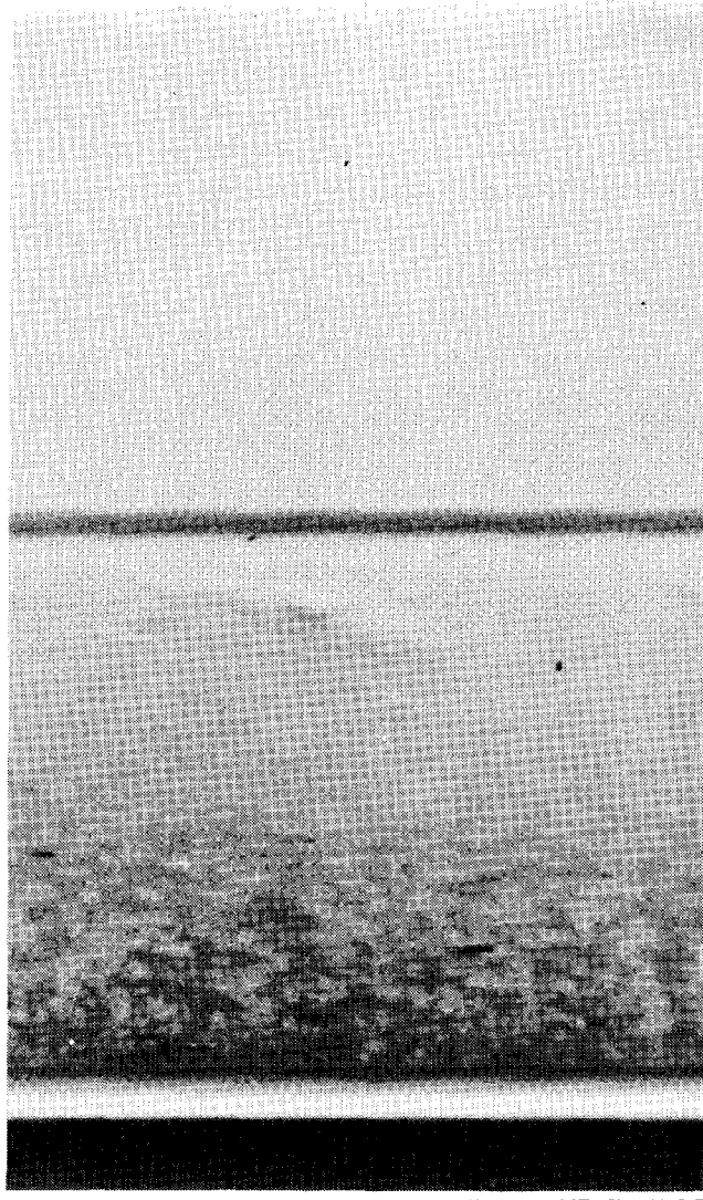
FIG. 4—TWO LB PER GAL. OF 20-40 MESH SAND IN 40 LB PER 1000 GAL. OF POLYMER
