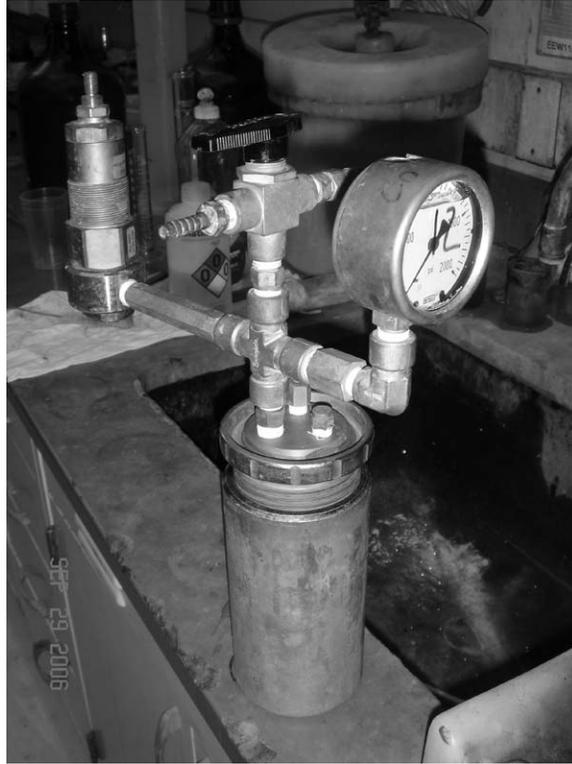
Figure 8—Testing Cell for the H<sub>2</sub>S and CO<sub>2</sub> Degradation Experiment
