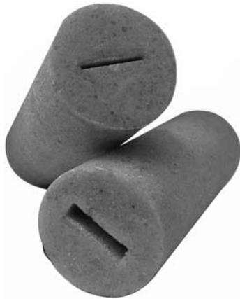
Figure 5—Synthetic Core with Created Fracture
