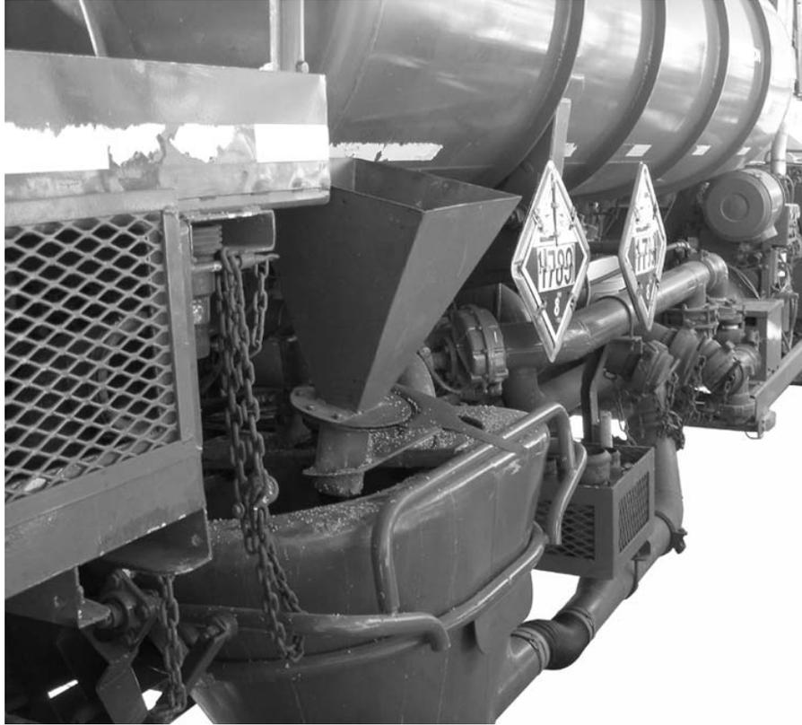
Figure 10—CLAM with CSC Injector
