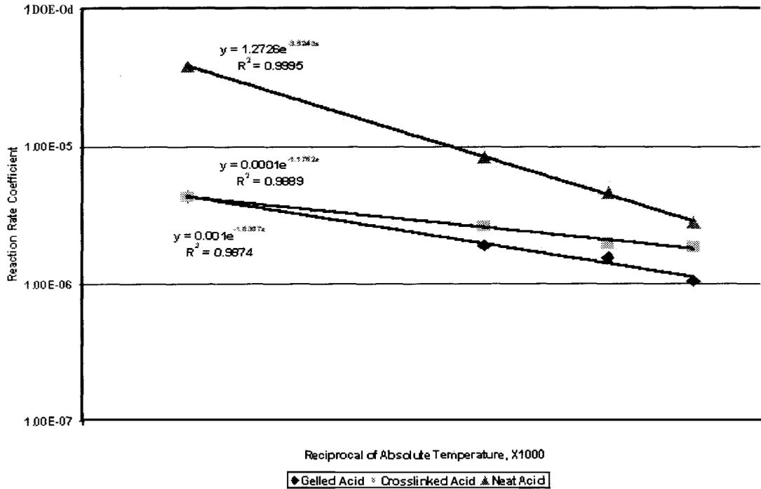
Figure 4 - Plots of Reaction Rate Versus the Reciprocal of Temperature (Absolute) for Neat, Gelled and Crosslinked (XLA-III) Hydrochloric Acid Reacted on Core Samples of Middle Eastern Limestone - The equation for the exponential trend of the data and the statistical coefficient are included. The resultant parameters are listed in **Table 8**.
