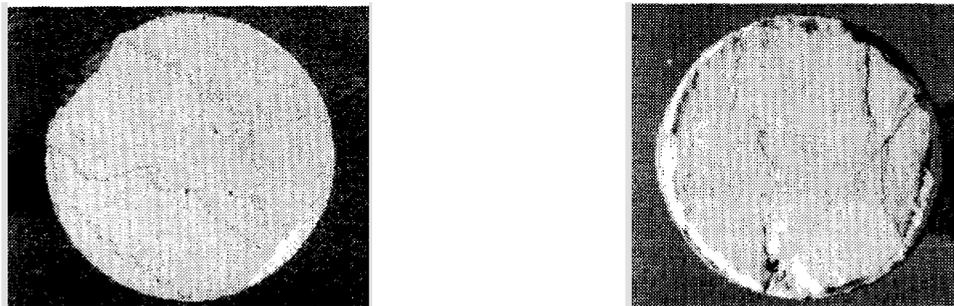
Figure 5 - Stylolites (black irregular lines) are evident in the North Sea chalk sample. The sample is hard and dense. The etched plug (right) exhibits relief along stylolite surfaces. Usually bitumen or clay is concentrated along these pressure solution features.
