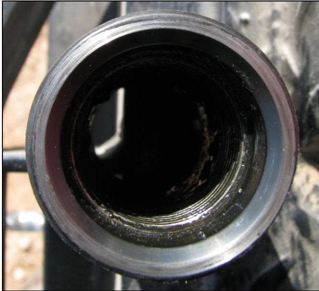
Figure 11 – Defective Coupling Identified by SmartTong SM
