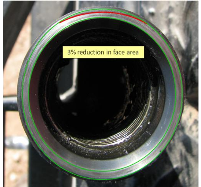
Figure 12 – Coupling Face Defect highlighted
