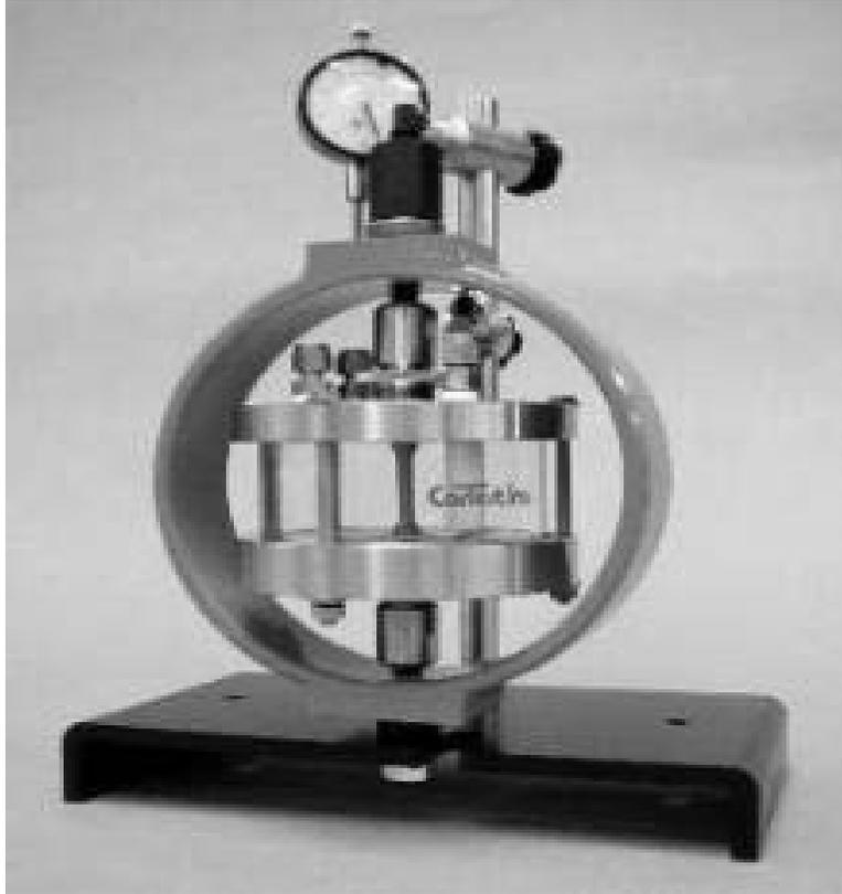
Figure 2- TM01-77 Test Apparatus
