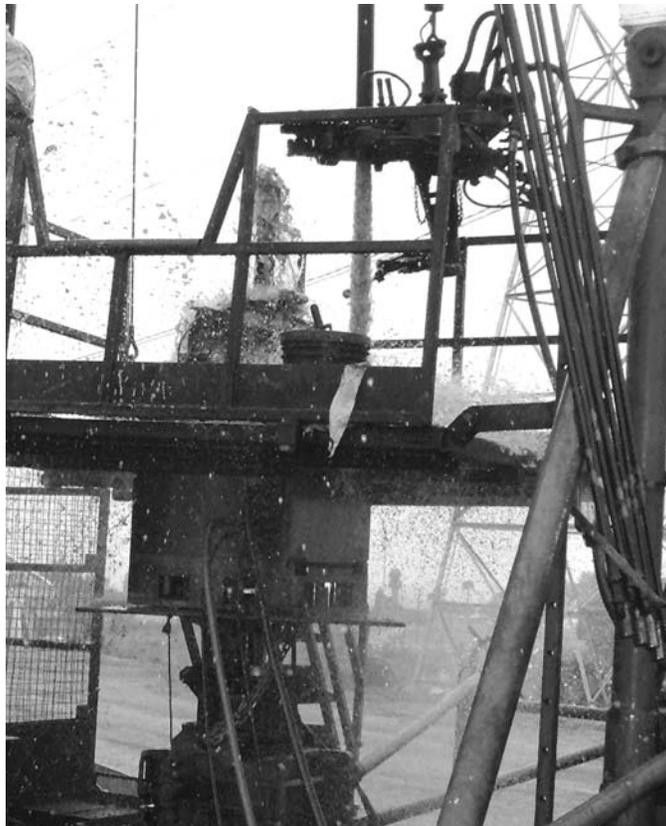
Figure 4a – Tubing Analysis During a Wet String Pull
