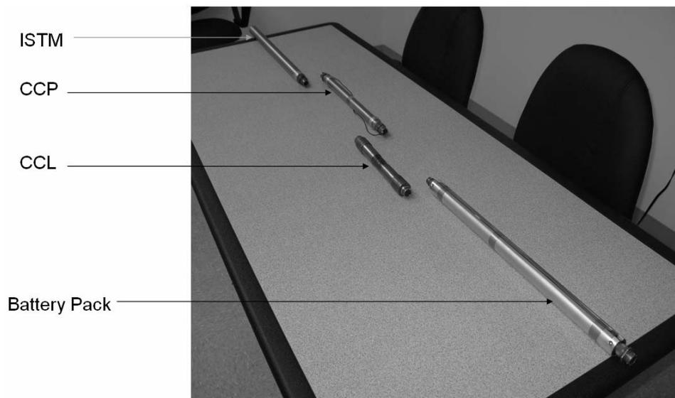
Figure 5 – Deviation Profile Tool Components
