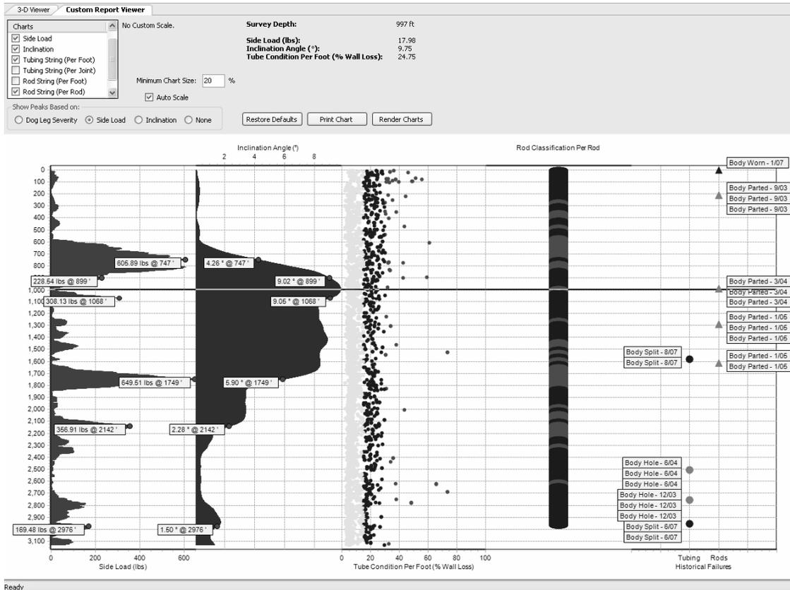
Figure 11 – Details of Wear and High Side Load Zones
