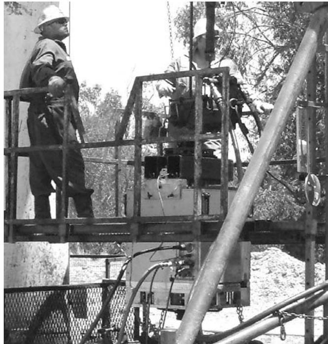
Figure 4 – RFSP Rigged Up During a Sucker Rod Analysis
