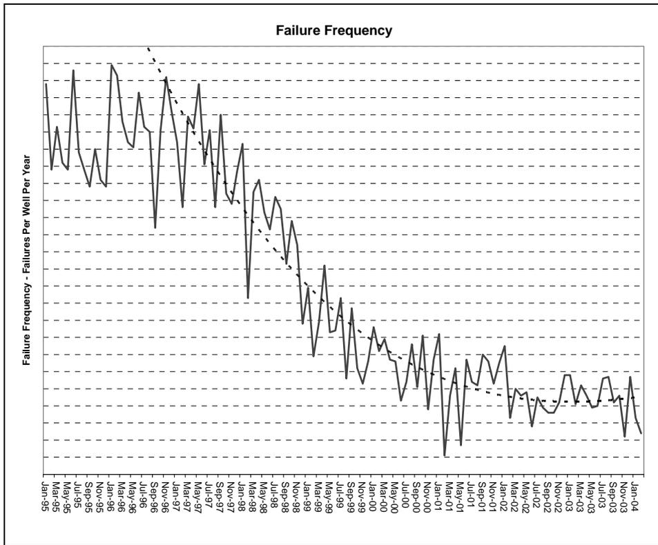
Figure 1 – Rod Pumped Well Failure History in a Large Permian Basin Field
