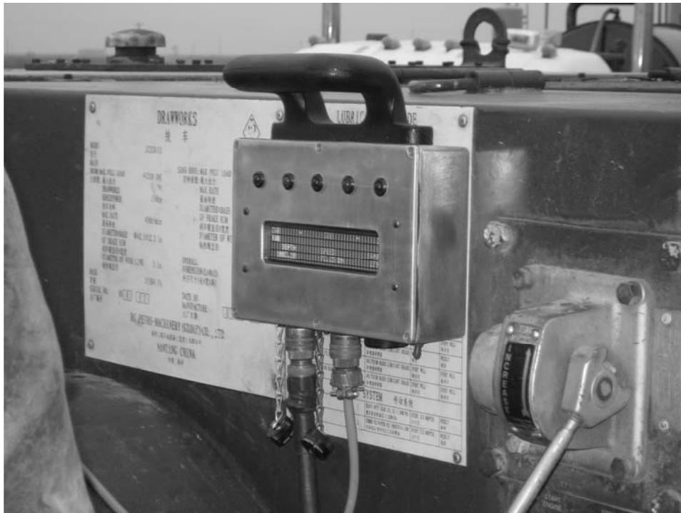
Figure 6 – Pulling Unit Operator's Remote Depth Display
