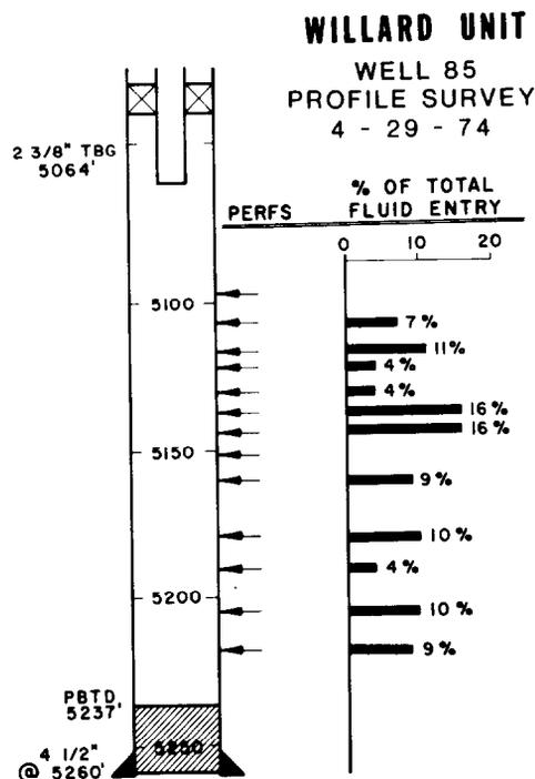
FIGURE 4—PHASE I WELL 85 WATER INJECTION PROFILE.
