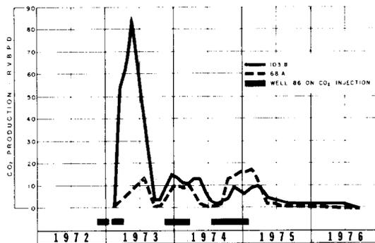
FIGURE 6—PHASE I WELLS 68A AND 103B CO<sub>2</sub> PRODUCTION.
