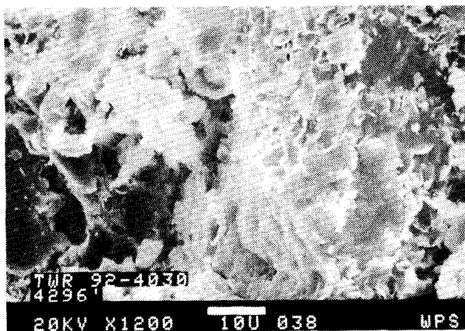
Figure 3 - Crenulated mixed-layer chlorite/smectite is seen at the right-center, coating a quartz framework grain. Illitic clays are also visible-at left-on a grain surface.
