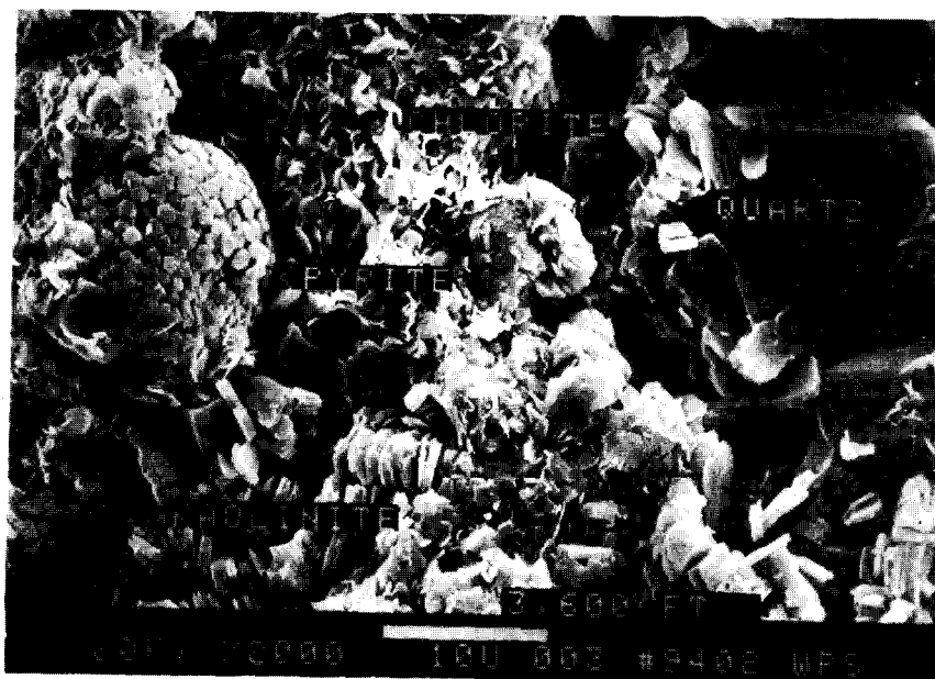
Figure 5 - Under 2000x magnification, kaolinite and chlorite clays are shown along with a pyrite frameboid. A secondary quartz overgrowth indicates at least partial cementation by quartz. Atascosa County, 3600'.
