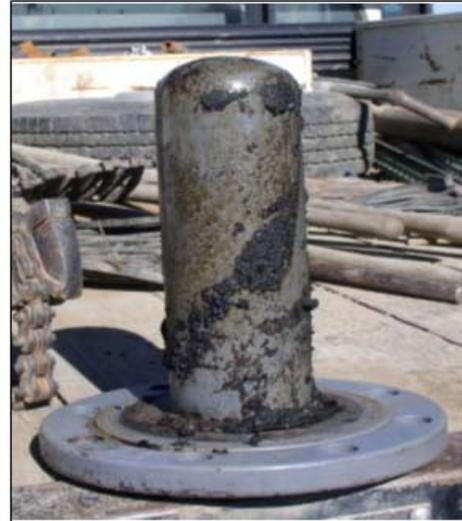
Figure 14 - Internal bluff body showing spiral of paraffin deposit after downhole hot water treatment. (Ref. 12)
