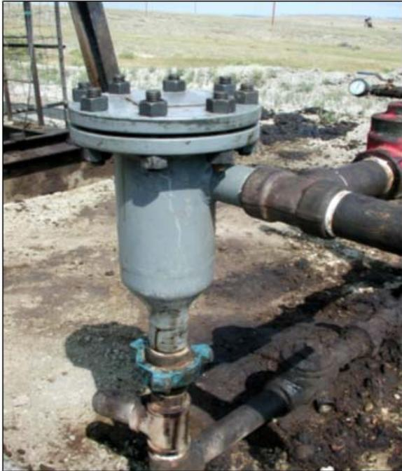
Figure 13 - New development of SX tool shows flanged back plate to aid in internal cleaning. This new tool is now the SX-P for surface paraffin mitigation. (Ref. 12)
