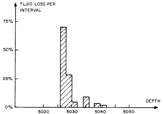
FIGURE 10 — INJECTION PROFILE FROM TABLE 4 (INTERVAL METHODS)
