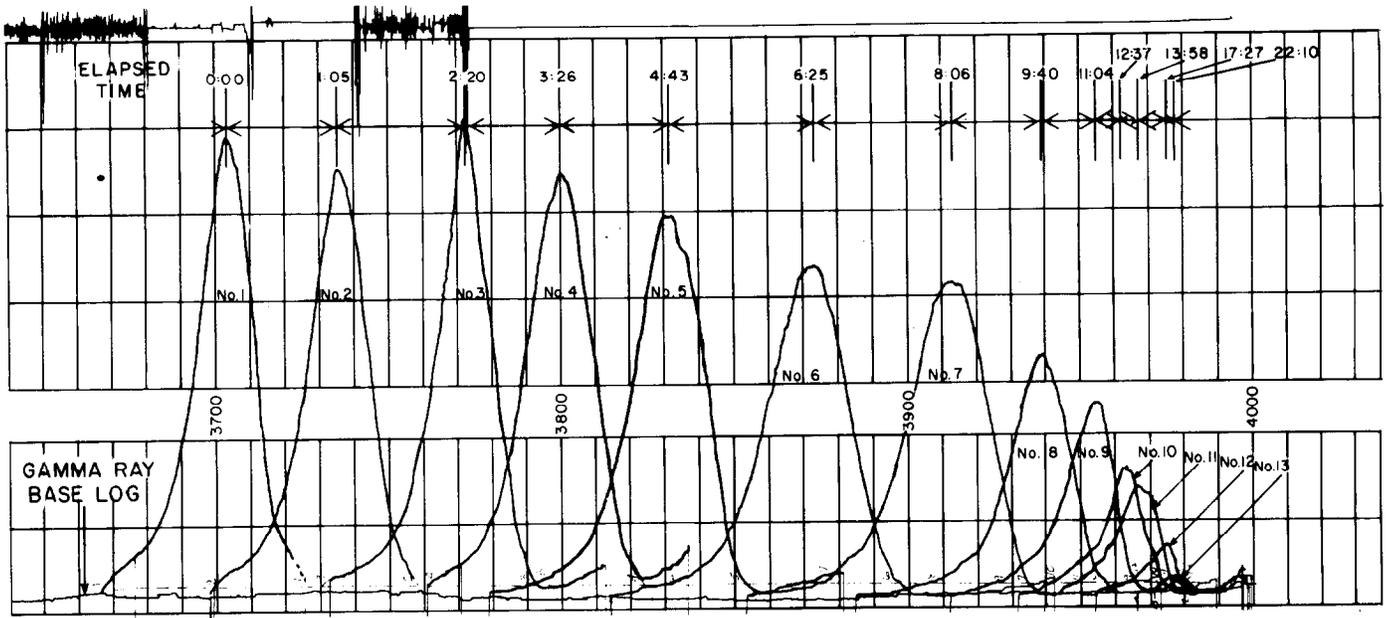
FIGURE 2 — TYPICAL TRACER LOSS LOG TRACES
