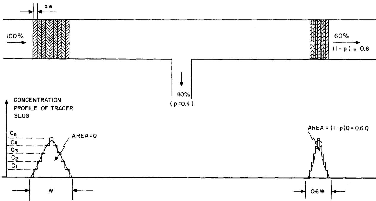
FIGURE 4 — SCHEMATIC SHOWING SYNTHESIS OF A REAL CONCENTRATION PROFILE FROM SLUG ELEMENT OF DIFFERENT TRACER CONCENTRATIONS
