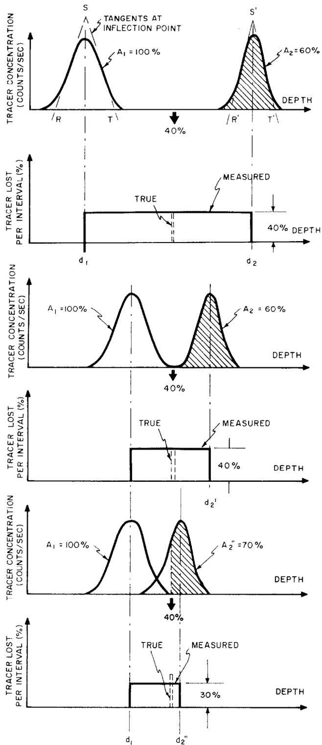
FIGURE 5 — EFFECT OF TRACER PROFILE PROXIMITY ON THE RESULTS FOR THE AREA METHOD FOR FLUID THROUGH A SINGLE PERFORATION
