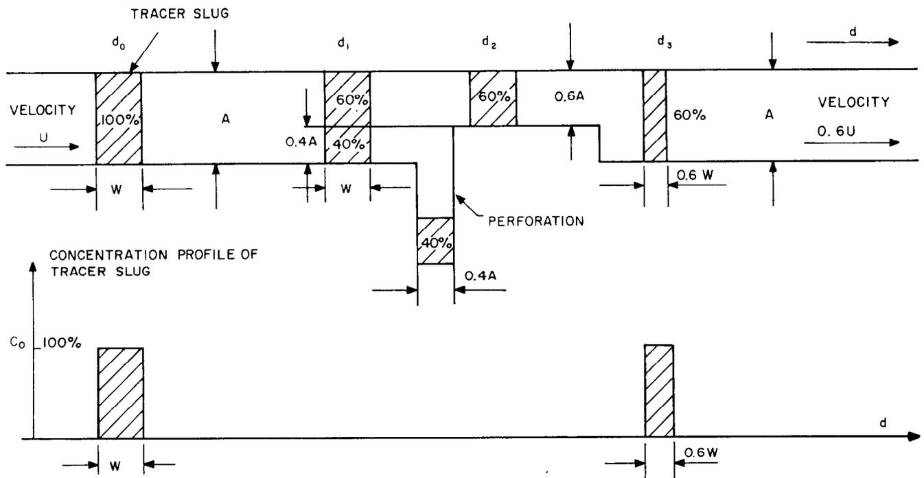
FIGURE 3 — SCHEMATIC ILLUSTRATING THE REDUCTION IN LENGTH OF A TRACER SLUG AS IT PASSES A PERFORATION
