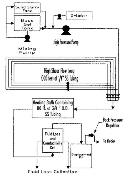
Figure 4 - Fluid preconditioning loops and dynamic fluid loss / conductivity apparatus
