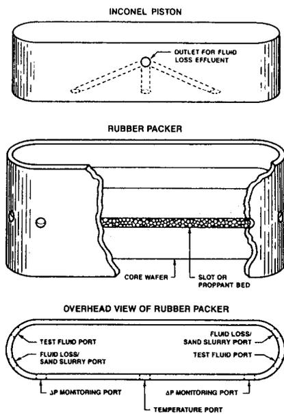
Figure 3 - Schematic showing one of the two pistons and a cutaway view of the core wafers inside the packer of the conductivity/ fluid loss test cell used
