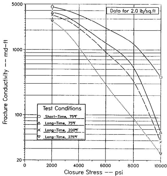
Figure 1 - Conductivity data for 20/40 Ottawa sand showing measured values from short-time test procedures to be overestimated
