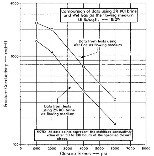
Figure 8 - Conductivity vs stress for 20/40 Ottawa sand in the presence of filter cakes from a crosslinked HPG gel
