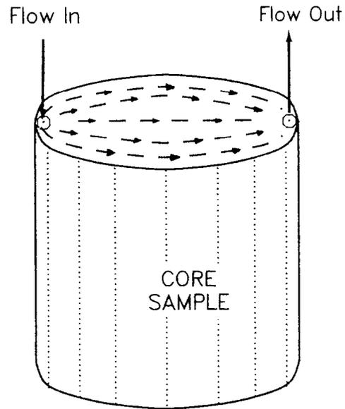
Figure 2 - Probable flow streamlines inside the proppant pack in a cell where cylindrical core with a proppant pack on top is held in a Hassler sleeve type cell
