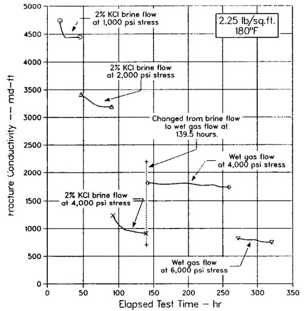
Figure 6 - Conductivity vs time for 20/40 Ottawa sand in the presence of filter cakes from a polymer emulsion fluid using 2% KCl brine flow then wet gas flow
