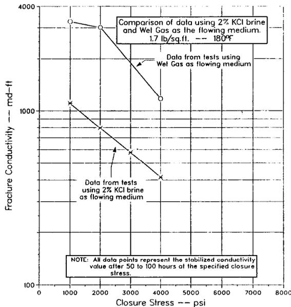
Figure 7 - Conductivity vs stress for 20/40 Ottawa sand in the presence of filter cakes from a linear HPG gel (40 lb per 1000 gal.)
