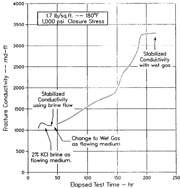
Figure 5 - Conductivity vs time for 20/40 Ottawa sand in the presence of filter cakes from a linear gel system containing 40 lb HPG per 1000 gal.
