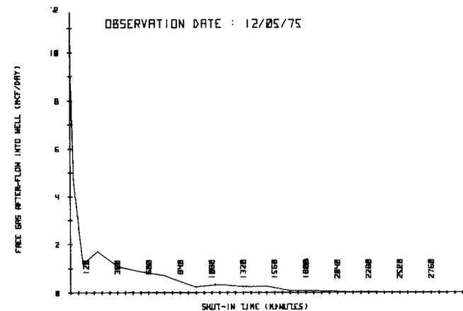
FIG. 14—FREE GAS AFTER-FLOW VS SHUT-IN TIME
