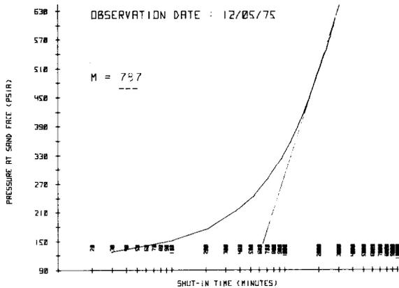
FIG. 17—MID-PERF PRESSURE VS LOG (T) EVALUATION OF KH
