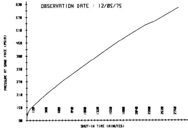
FIG. 13—PRESSURE AT MID-PERF DEPTH VS SHUT-IN TIME
