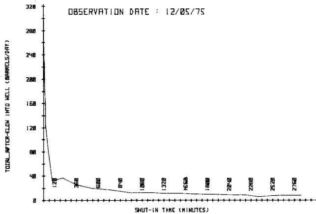
FIG. 16—TOTAL AFTER-FLOW VS SHUT-IN TIME
