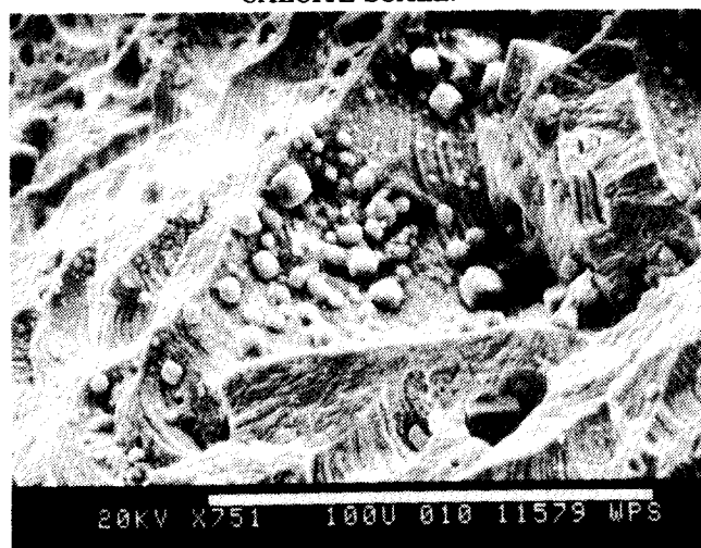
FIGURE 3—IRON SULFIDE SCALE SHOWING SMALL CUBIC CRYSTALS.
