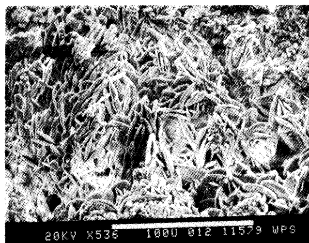
FIGURE 5—BARITE SCALE SHOWING "CRESTED BARITE" APPEARANCE.
