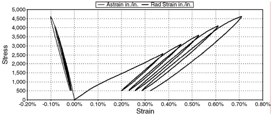
Figure 6—First Partial-cyclic Tests for Cement System 4
