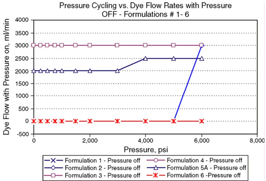
Figure 14—Fluid flow rates through the wellbore model with pressure off.
