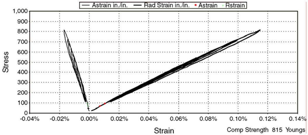
Figure 9—First Partial-cyclic Tests for Cement System 1
