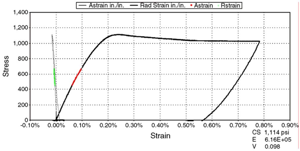
Figure 8—Stress-strain Curve for Cement System 1, Confined
