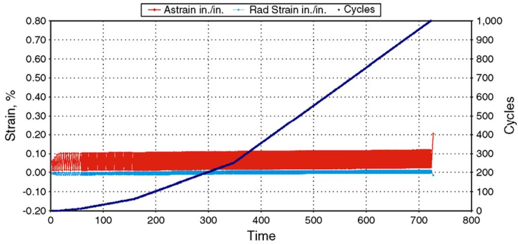
Figure 11—Cyclic Tests for Cement System 1
