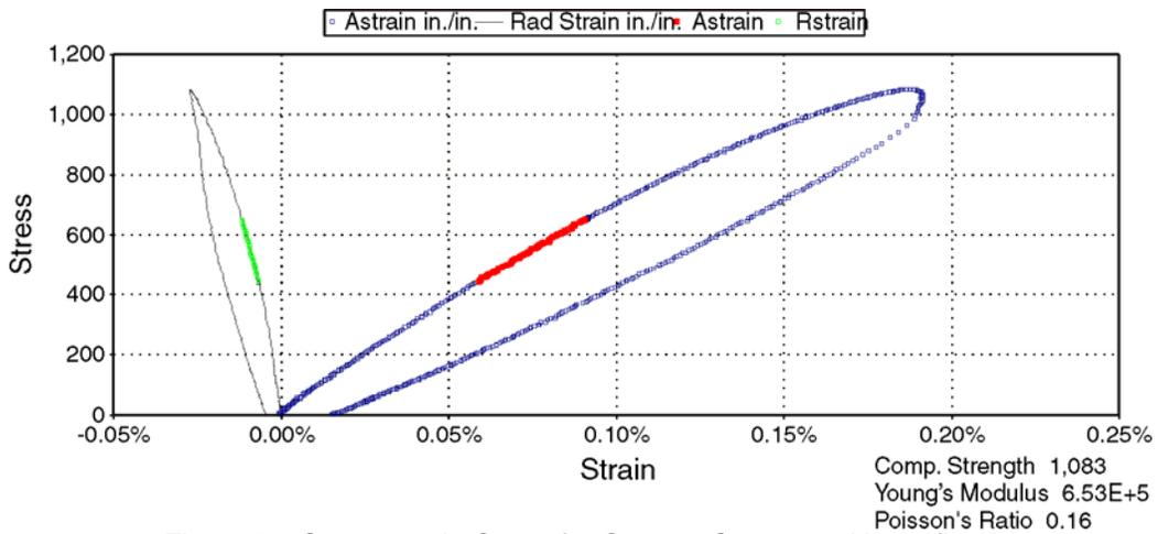
Figure 7—Stress-strain Curve for Cement System 1, Unconfined
