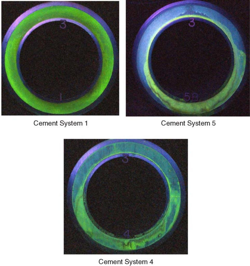
Figure 3—Photographs taken in UV black light of cut sections of wellbore models.
