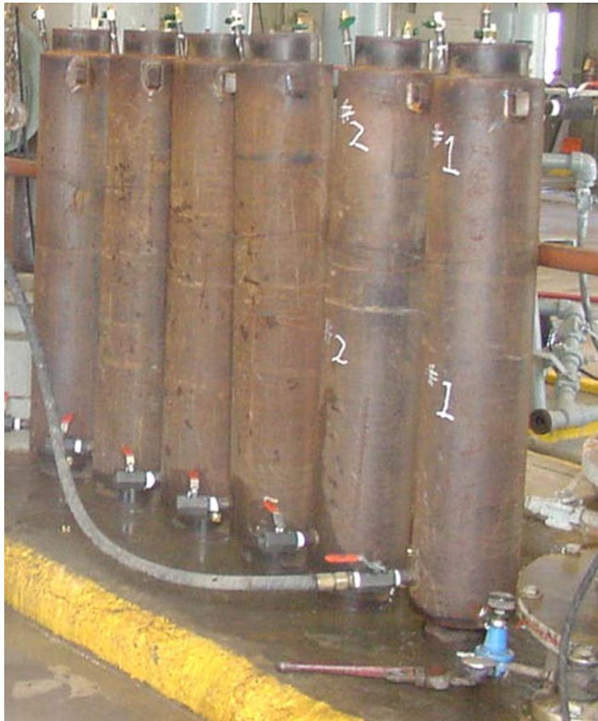
Figure 1—Pipe-in-Pipe Wellbore Model
