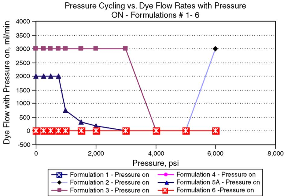
Figure 13—Fluid flow rates through the wellbore while the pressure is on.
