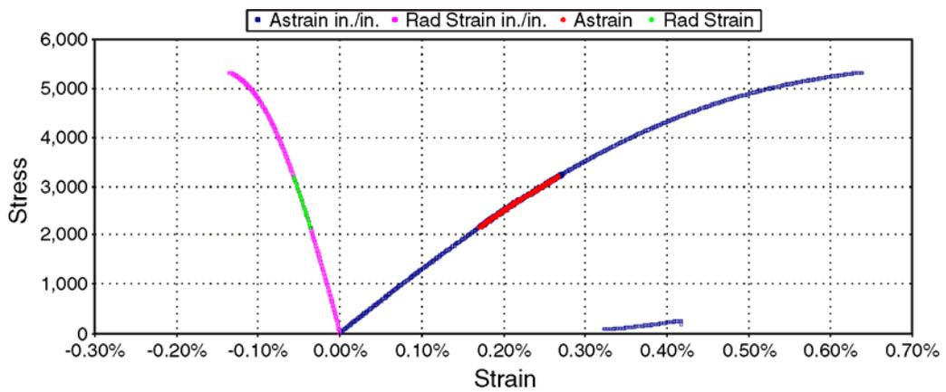
Figure 4—Stress-strain Curve for Cement System 4, Unconfined
