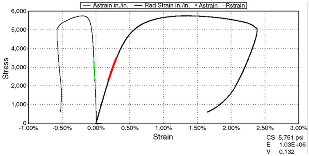
Figure 5—Stress-strain Curve of Cement System 4, Confined
