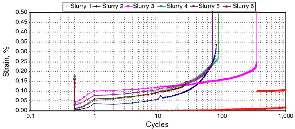
Figure 10—Plastic Strains of Various Cement Systems
