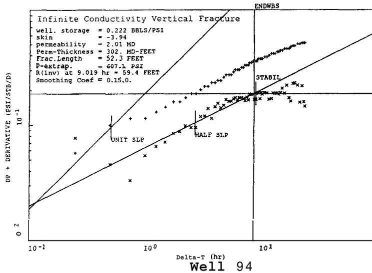
Figure 6 - Log-Log Plot of Pressure (+) and Pressure Derivative (x) for LLU 94 PFO Test. Derivative smoothing of 0.15 was required to observe reservoir features. Half-slope indicative of a fracture is present through about 3/4 log cycle of SI time. The  $x_f$  calculated is 52'.
