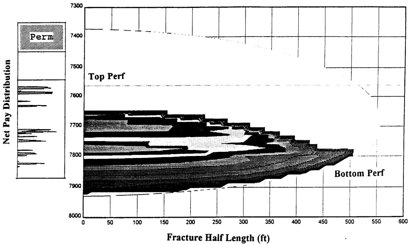
Figure 11 - Field Example 6 Offset Proppant Distribution
