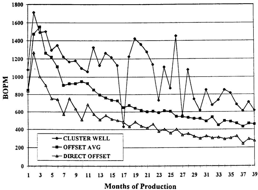
Figure 12 - Field Example 6 Cluster Well Production vs. Offsets
