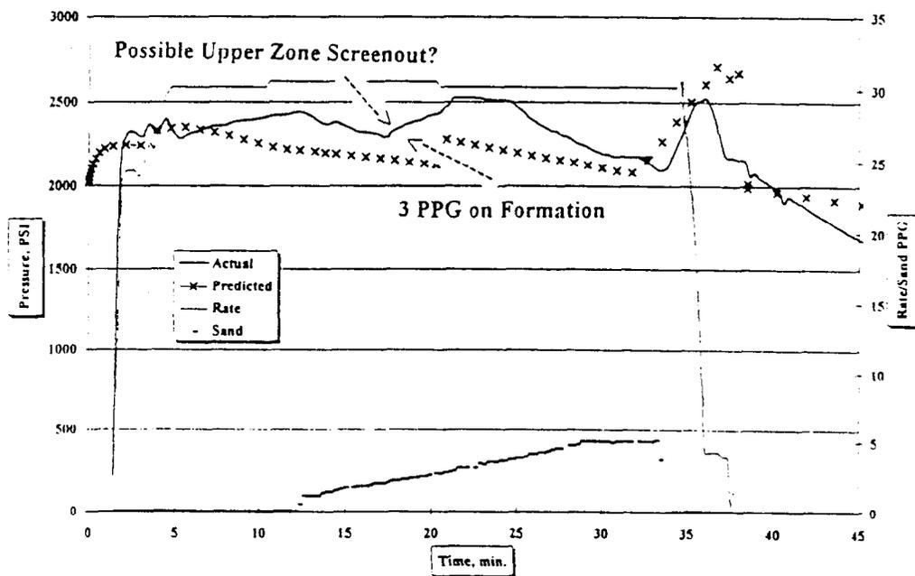
Figure 5 - Field Example 2 Surface Pressure Plot
