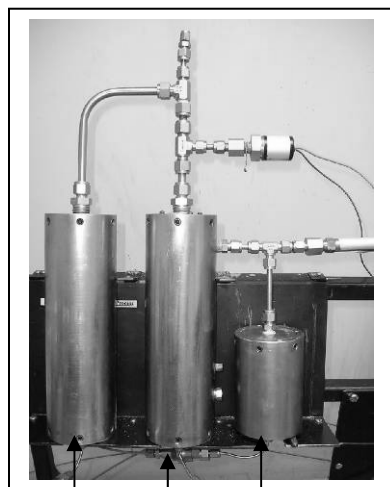
Figure 2 - Schematic of Impermeable Fracture Test Device The test apparatus consists of a mud reservoir (left cylinder, MR1), fracture cell (center cylinder, FC), and fracture-tip accumulator (right cylinder, MR2).
