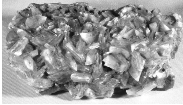
Figure 3 - Calcium Sulfate (Gypsum) Scale
