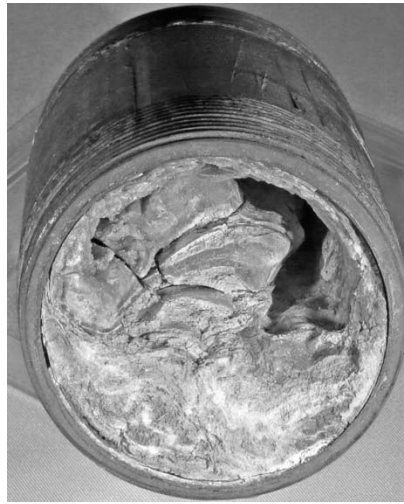
Figure 4 - Barium Sulfate Scale
