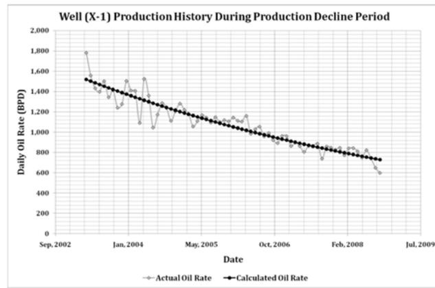
Figure 10- Well X-1, Decline Period Analysis Linear Plot. (Actual and Calculated Oil Rate)
