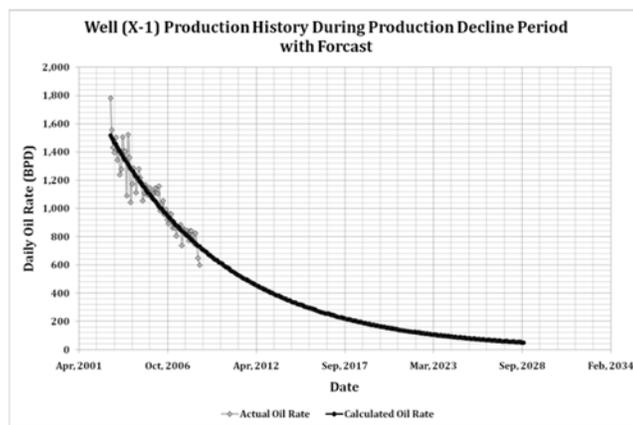
Figure 11- Well X-1, Decline Period Analysis with Forecast Linear Plot. (Actual and Calculated Oil Rate)
