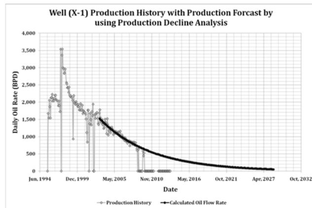
Figure 13- Well X-1, Production History with Production Forecast by using Production Decline Analysis Linear Plot. (Actual and Calculated Oil Rate)
