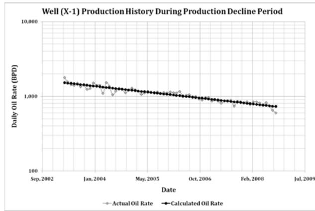
Figure 12- Well X-1, Decline Period Analysis Semi-log Plot.(Actual and Calculated Oil Rate)
