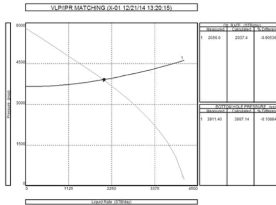
Figure 4- Well X01-1995; Nodal analysis by using Fancher VLP correlation after matching reservoir pressure.
