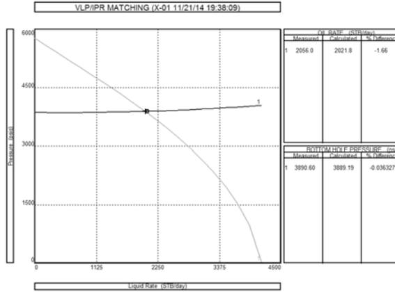
Figure 3- Well X01-1995; Nodal analysis by using Fancher Brown VLP correlation after matching VLP curve.
