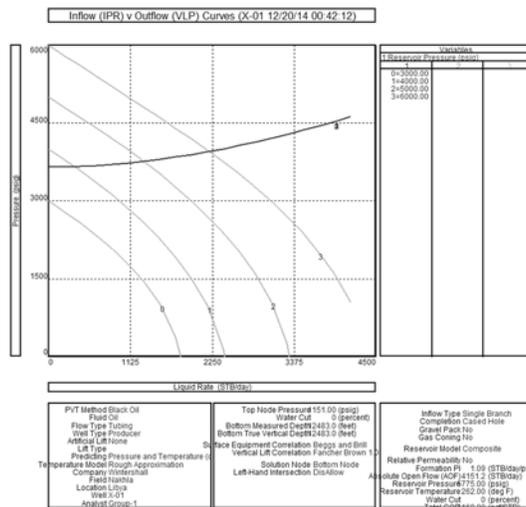
Figure 5- Well X01-1995; Sensitivity analysis to reservoir pressure by using Fancher Brown VLP correlation after matching.
