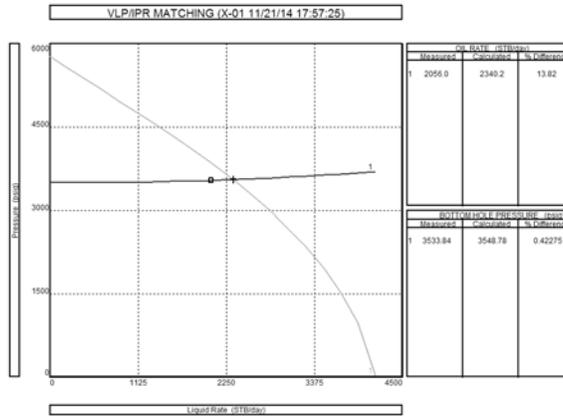
Figure 2- Well X01-1995; Nodal analysis by using Fancher Brown VLP correlation before matching VLP curve.
