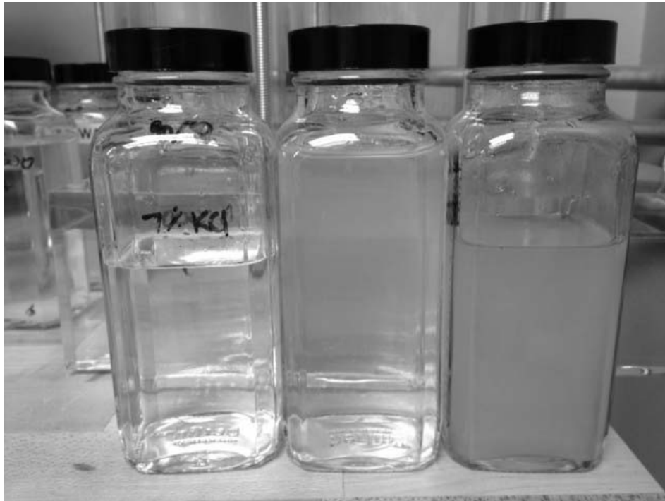
Picture 2 Effluent from a Sand/Clay Column Test Showing Clay Fines (From Left to Right, Minute Fines, Some Fines, Significant Fines).
