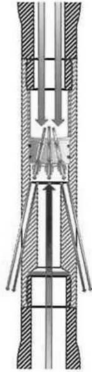
Figure 4 – Venturi Jetting Tool Cutout, power fluid pumped down tubing from surface out venturi jets, low pressure drop is generated inside the basket cavity
