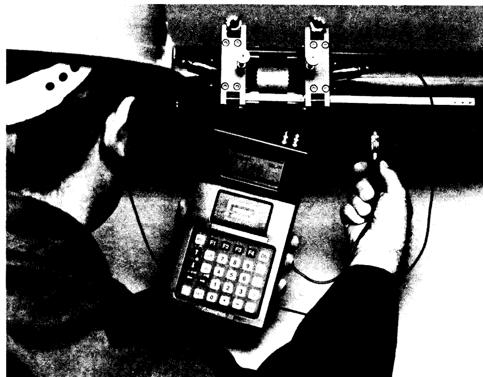
Figure 5 - Example of PT868, a portable clamp-on (or wetted transducer) battery-powered correlation detection flowmeter. It was programmed in 1992 to operate as a transit time instrument when it is temporarily operated as a thickness gage. In 1993, new programs are expected to extend its operating modes to include reflection. This will be a multipulse tracking mode, different from the usual Doppler flowmeters, but nevertheless responsive to the flow velocity of scatterers in the fluid. Technical capabilities for this instrument include storage capacity for 40,000 data points, 20 site location parameters, on-line pipe tables, and graphic or alphanumeric LCD display.
