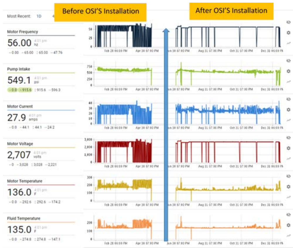
Figure 11. Sensor parameters AFTER Guardian Shield Installation - Parker JE 5
