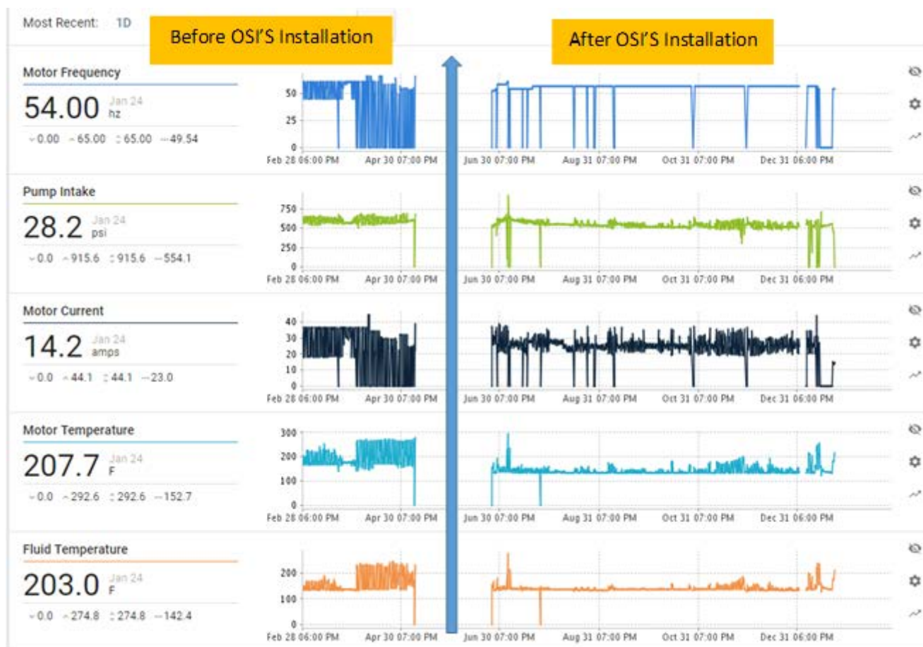
Figure 14. Sensor parameters AFTER Guardian Shield Installation – Cousin Willard 450 4H
