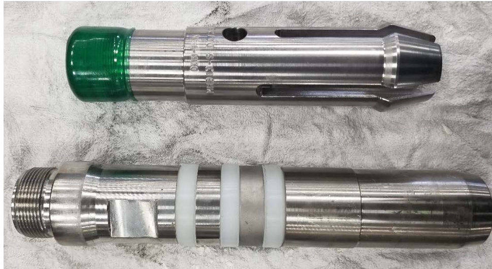
Figure 8 shows a side-by-side comparison of seating assemblies. The mechanical style seating assembly (top) is for high temperature applications while the cup style assembly (bottom) is the more common selection
