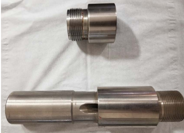
Figure 10 shows an example of the external seat plug and top plunger adapter used in Sand Diverter pump applications
