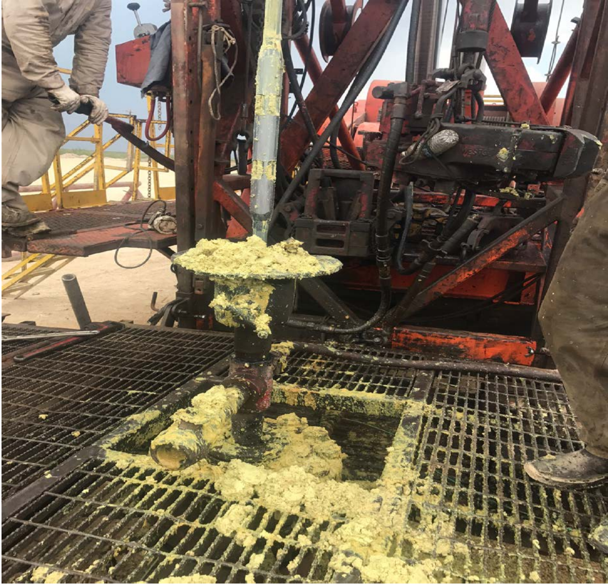
Photo 2 Illustrates paraffin stripping while pulling out with rods on a typical workover in Bloxom.
