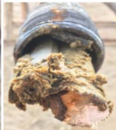
Photo 12 Shows the paraffin level in the Crystal #1 prior to the Enercat installation.
