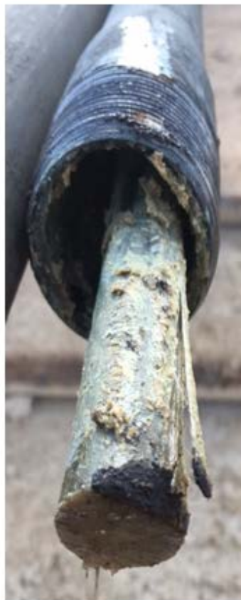
Photo 12 Shows the paraffin level in the Crystal #1 prior to the Enercat installation.
