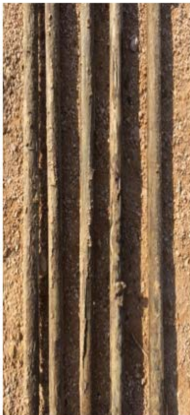
Photo 12 Shows the paraffin level in the Crystal #1 prior to the Enercat installation.
