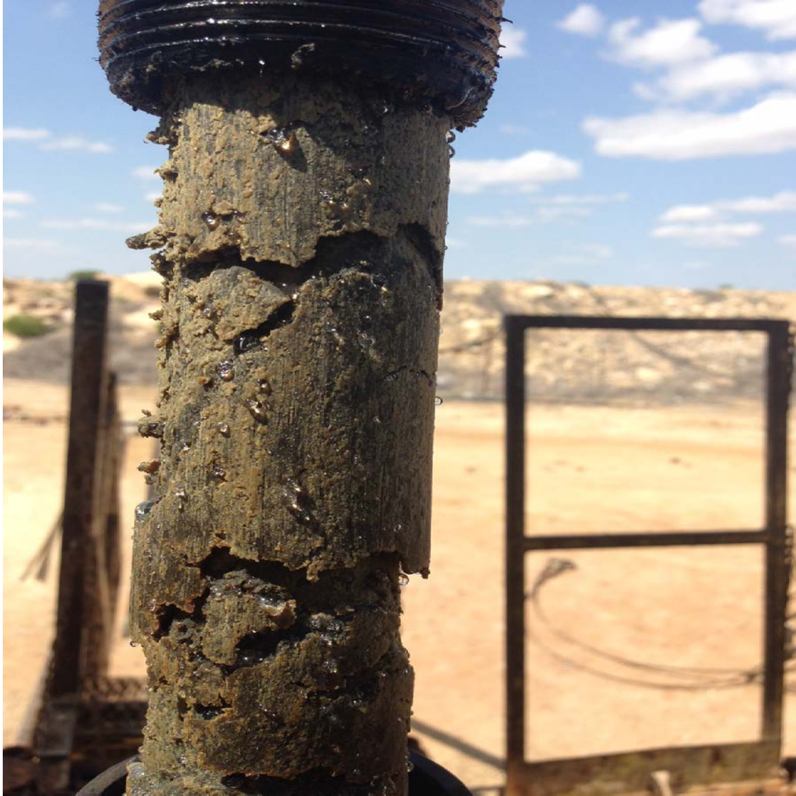
Photo 3 Illustrates paraffin occupying every void space between the rod and tubing during a recent workover.
