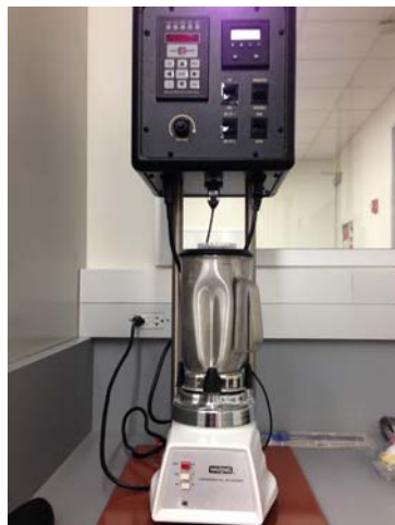
Figure 1– Fracturing Fluids Blender
