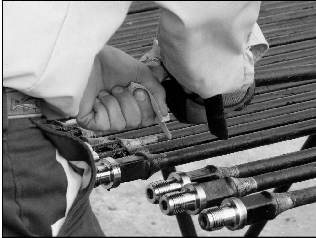
Figure 1 – Proper cleaning of components is critical to obtaining good CD and connection preload
