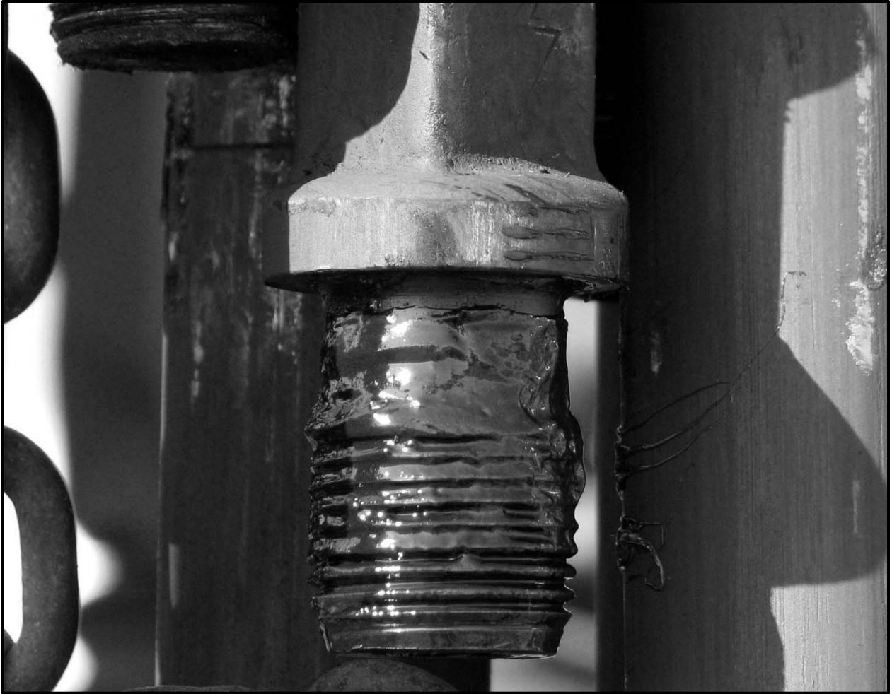
Figure 9 – Wellbore fluid inside the connection indicates separation of the faces and loss of preload. This is a failed condition and should not be accepted as normal.
