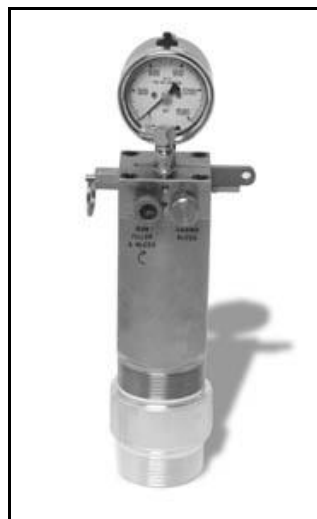
Figure 4 - Compact Gas Gun Modified (as shown by the engraving) with Special Microphone for use in Hazardous Areas
