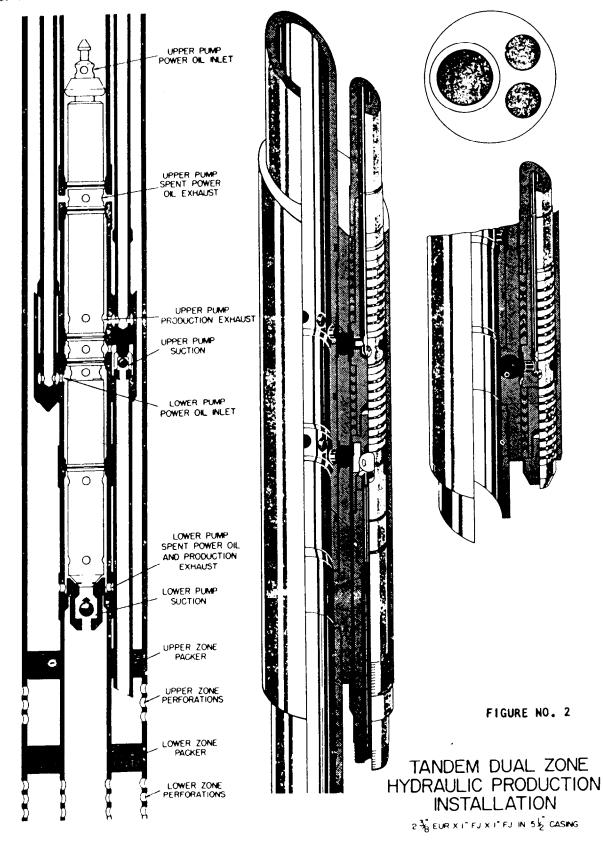
man zone at about 8000 ft. The bottom hole assembly for the hydraulic pumps is immediately above this packer.
