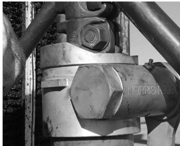
Figure 12 – Norris slow gear rotator with polished rod clamp lock-in System
