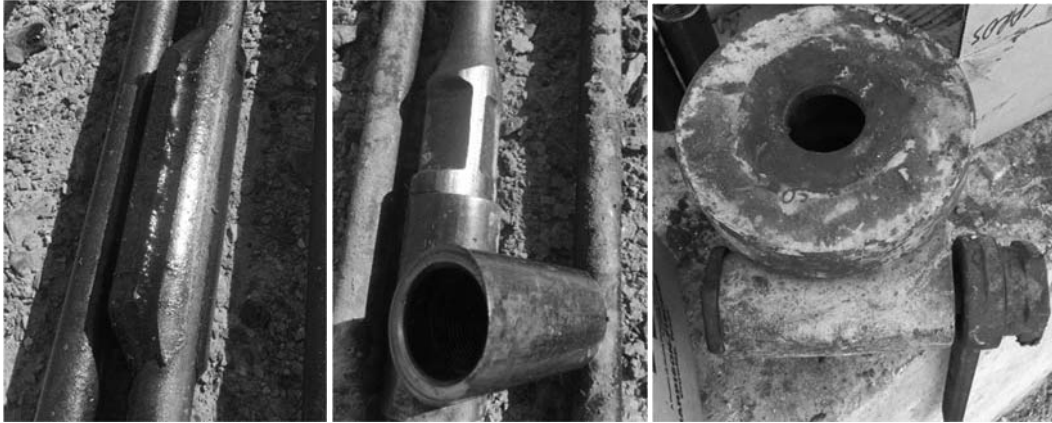
Figure 10 – One-sided rod string wear with friction-dependent rod rotators
