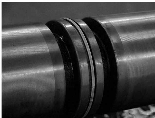
Figure 24: Motor Radial Thrust Bearing: White out, blue in – heating
