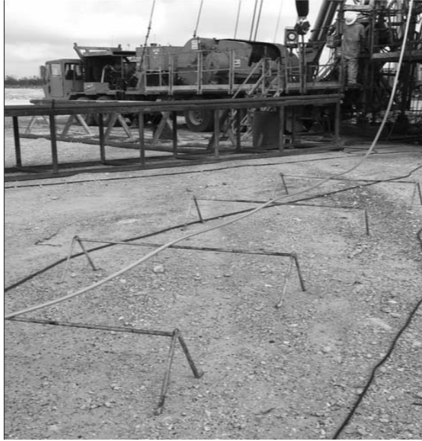
Figure 14: Cable sills/supports (adequate number)
