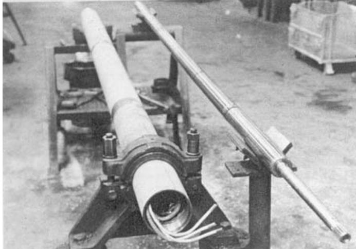
Figure 22: Motor in Shop: Head and rotor stack removed
