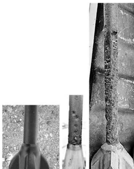
Figure 2 – Effect of turbulence after guides, a) Tenflow, b) Guide A, c) Guide B. Guides a and b were working the same time in same well
