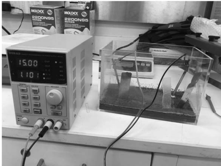
Figure (2) Applying a voltage across saltwater mud
