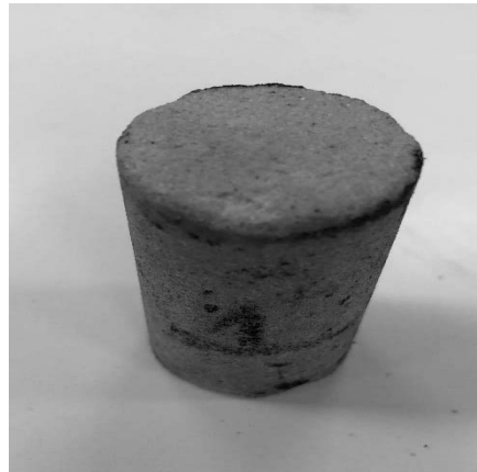
Figure (8) Shows Damaged Bernheimer sandstone core caused by 25% of Liquid Block 40F
