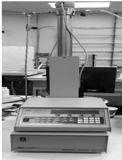
Figure (2): Experimental model Syringe Pump: main apparatus used for dynamic filtration
