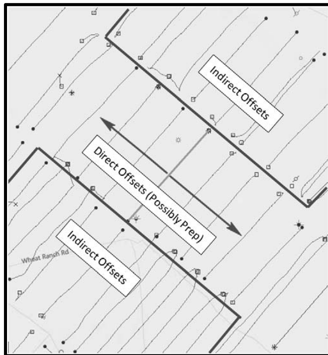
Figure 6: Direct vs. Indirect Offset Wells
