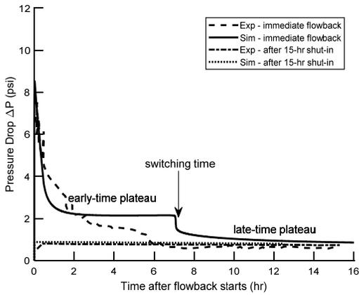
Figure 4 – Effect of shut-in and its timing on drawdown during flowback
