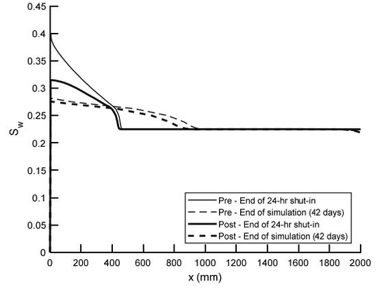
Figure 6a – Evolution of water saturation profile: shut-in pre-flowback
