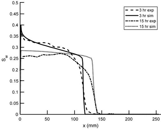
Figure 3 – Regained  $k_{ro}$  history match: experiment vs. modeling for immediate flowback and shut-in case [7]
