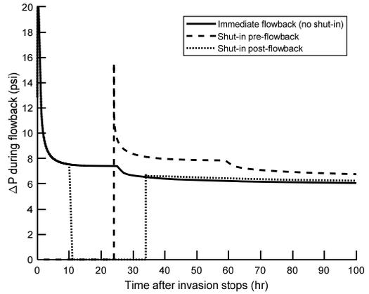
Figure 5 – Effect of shut-in and its timing on the restoration of  $k_{rO}$
