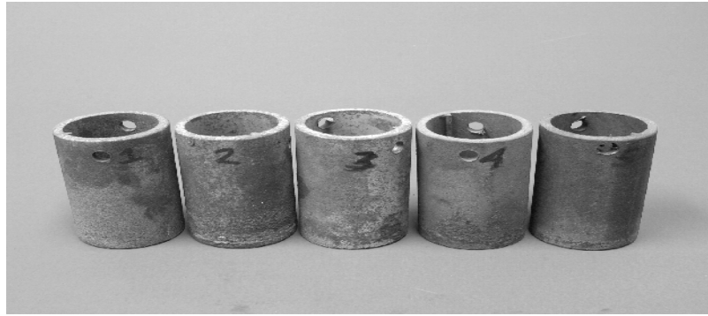
Figure 5 - Treated Coupons After 21 Day Incubation At Atmospheric Conditions
