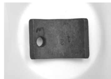
L80 Coupon Treated With 12vol% Environmentally Friendly Pickling Fluid + 25vol% Terpene Based Solvent
