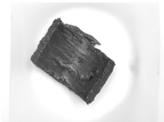
L80 Coupons Coated With Pipe Dope Before Testing
