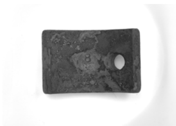
L80 Coupon Treated With 15% HCl Acid + 25vol% Terpene Based Solvent
