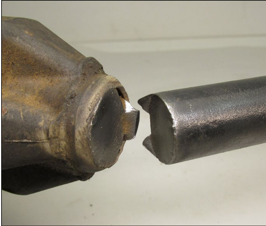
Figure 10 – Rod break occurring at end of molded guide section with flexural loading conditions.
