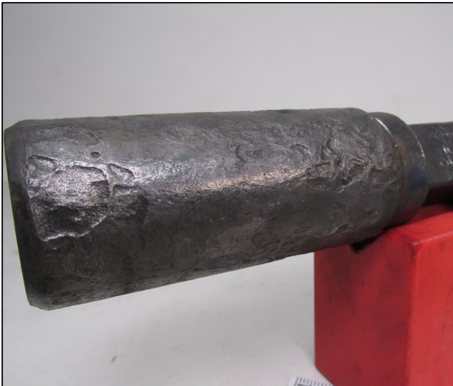
Figure 11 – Significant corrosion attack on T-coupling observed.
