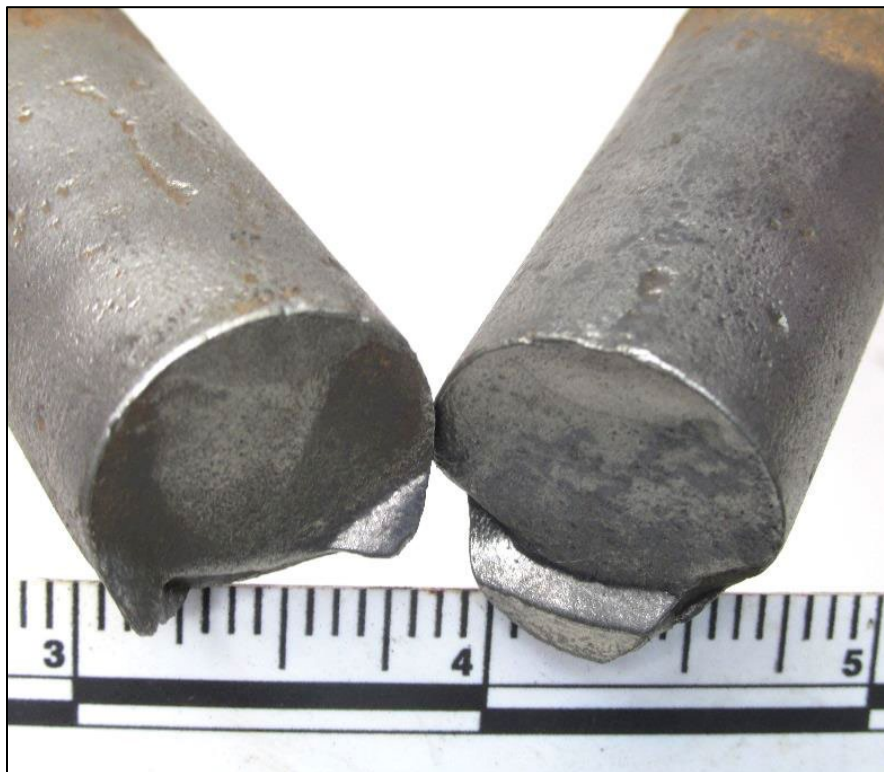
Figure 9 – Rod break presenting corrosion at initiation and flexural loading conditions (dual shear-lips).
